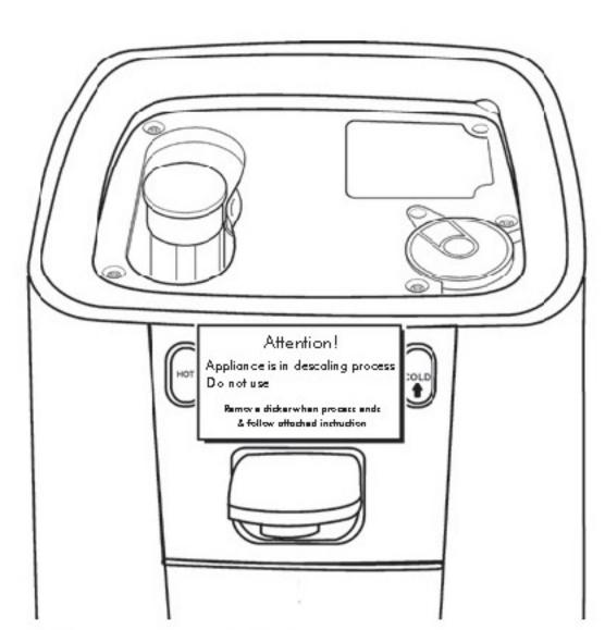
10 Place a 5 liter container under the spout, replace the filter and push until you hear a click.
