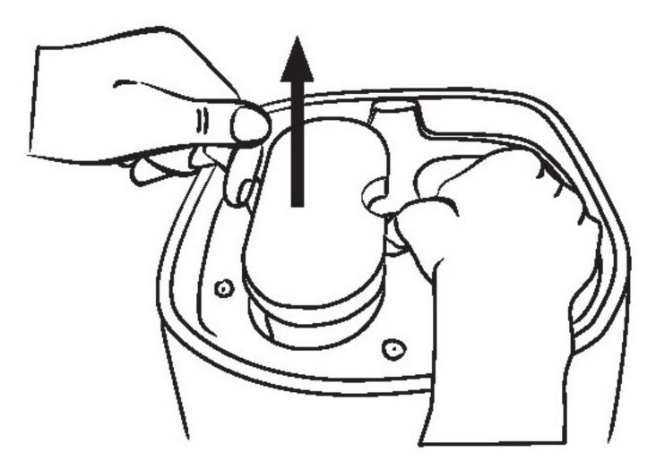
Insert the capsule into the filter's position (in any direction) until you hear a click.
