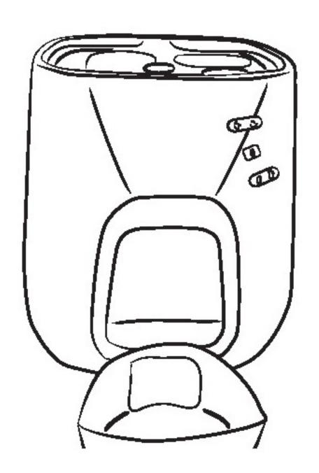
Press the PUSH button and pull the filter upwards using the extraction band.
