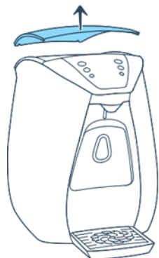
1. Remove the top panel.
